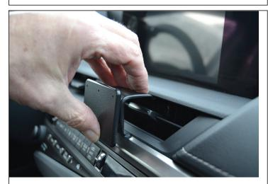
3. Flex the top of the mount down and hook the top edge under the top edge of the vent frame.
